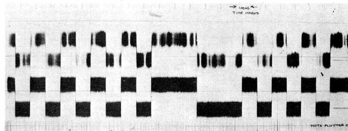
Fig 8. The letters 5B of 5B4CY as received by ZS6PW at 1845gmt on 30 January 1979 simultaneously on 50.498 and 28.220MHz. Note that the 50MHz pulse is 2ms behind the 28MHz pulse, which is a function of the keyer
